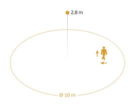
Possible mounting height: 2,00 m – 4,00 m Orange: radial and tangential
